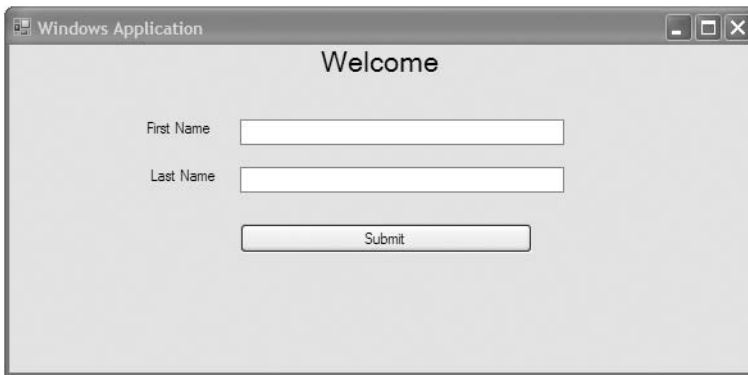
Figure 14-14. The effect of the Anchor property setting Top, Left, Right on a resized form
